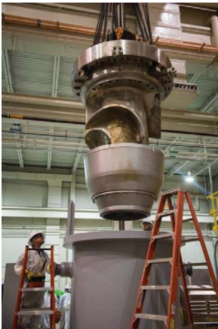
A newly refurbished reactor coolant pump is prepared for shipment.
