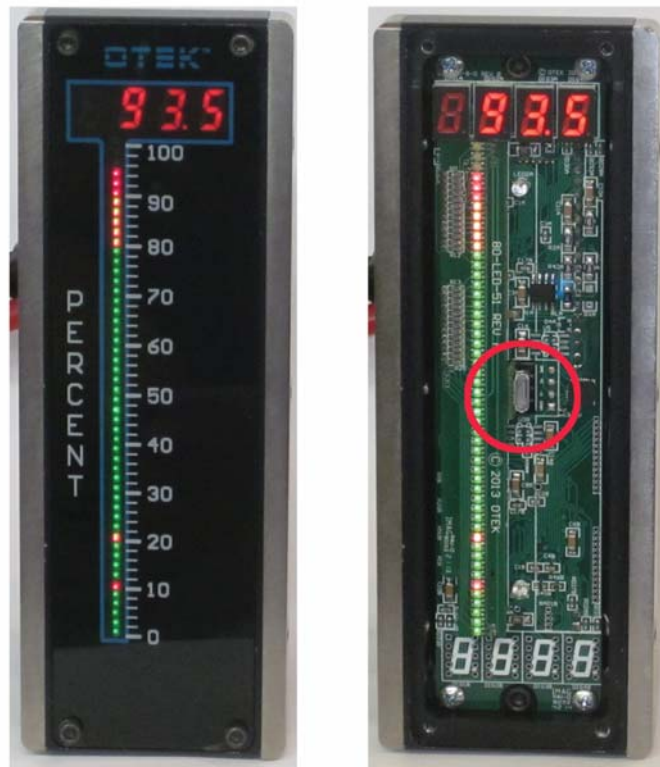
Figure 1: OTEK NTM-9 Digital Panel Meter and Bargraph. Note the access to the serial I/O port is behind the faceplate which requires removal of 4 screws in order to access the port. Access only from the rear of the instrument, behind the control panel, is also available.
