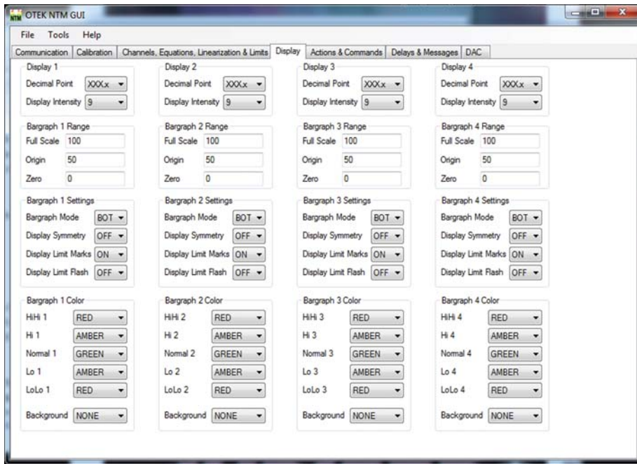
Figure 2: Screen shot from the Free OTEK GUI User Software illustrating the various configuration settings that are available to the user for personalization in the field.
