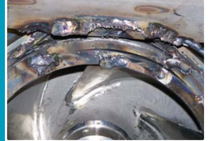
Rotor was damaged due to pump running dry for approximately 30 minutes.
