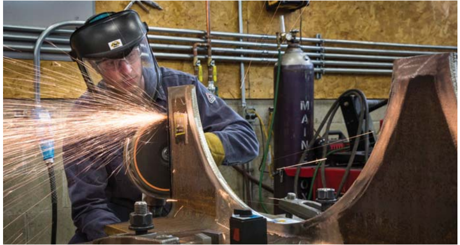
An air tank mid-frame is prepared for fabrication by a Westinghouse fabrication mechanic.
